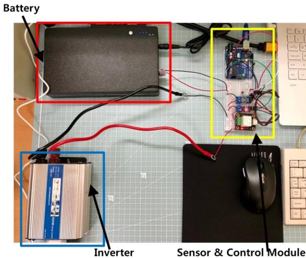
Fig. 4. SMC algorithm test system.
