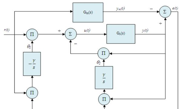
Fig. 6: Model Reference Adaptive Controller using Lyapunov’s Rule [17]
