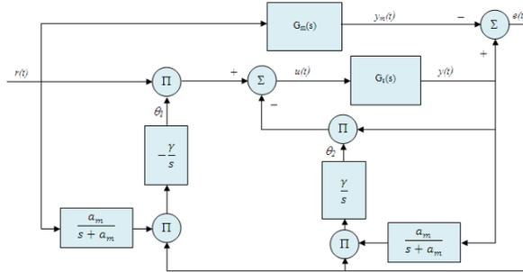
Fig. 7: Model Reference Adaptive Controller using the MIT Rule [17]
