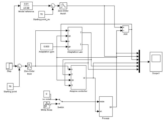
Fig. 8: MRAC Structure in Simulink Block
