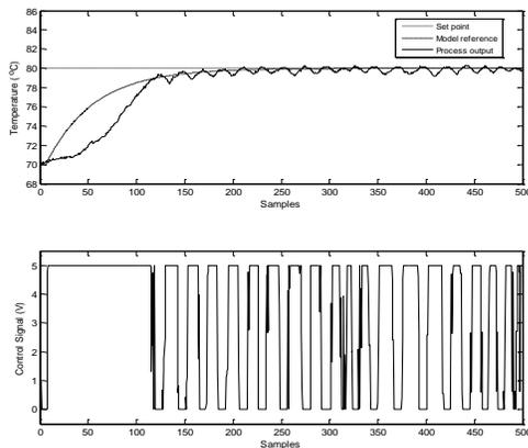
Fig. 17: Process Output and Controller Signal of Real-time MRAC-Lyapunov
