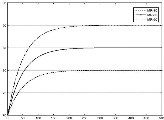
Fig. 4: Model Reference Curves for 80°C, 85 °C, and 90 °C Temperature Regulation
