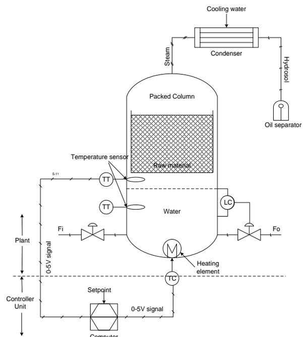
**Fig. 2:** Steam Distillation Process for Essential Oil Extraction
