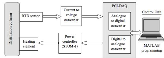
**Fig. 1:** Block diagram of steam distillation plant, computer and interface.
