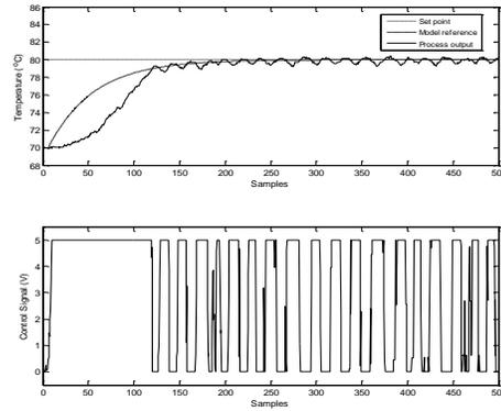
Fig. 18: Process Output and Controller Signal of Real-time MRAC-MIT Figures 17 and 18 illustrate the performance of optimal MRAC-Lyapunov (A6\_RT) and MRAC-MIT (B6\_RT) controllers with their control signals respectively. From the figures, both controllers were capable in terms of tracking model reference approximately at the 200th samples until reaching a steady state with oscillation at the set point.
