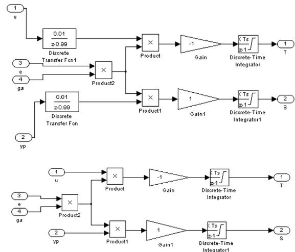
Fig. 9: Simulink Model of Adaptation Law MRAC Structure: (a) MIT Rule, (b) Lyapunov’s Theorem
