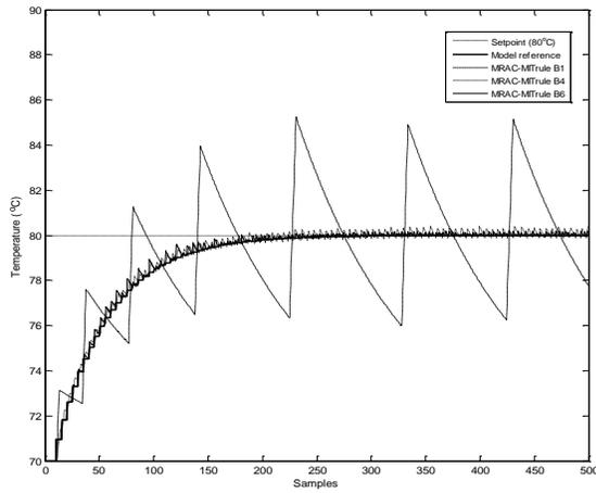
Fig. 12: Simulation of MRAC based on MIT-rule Scheme
