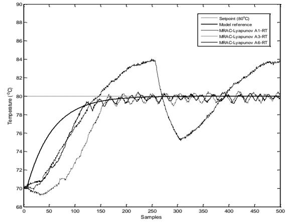
Fig. 13: Process Output using Real-time MRAC–Lyapunov Control Scheme
