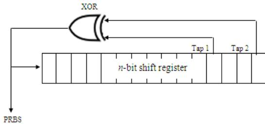
**Fig. 3:** Realization of PRBS tapping at LFSR with XOR gate at the feedback.
