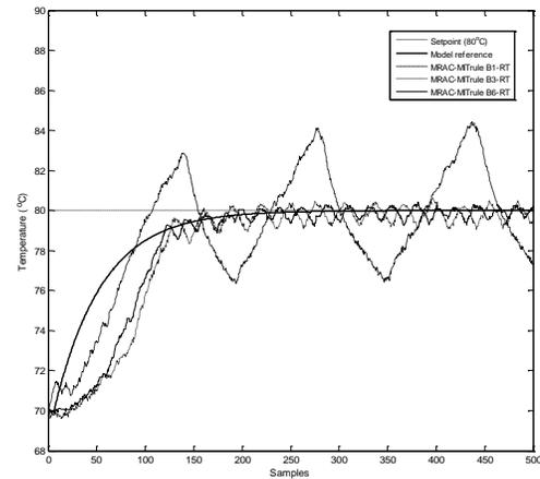
Fig. 14: Process Output using Real-time MRAC–Lyapunov Control Scheme
