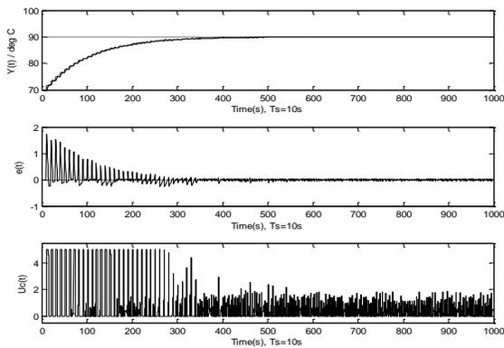
**Fig. 10:** Temperature response, Error and Controller Output when value of AG= 0.003 and IG=1.0.
