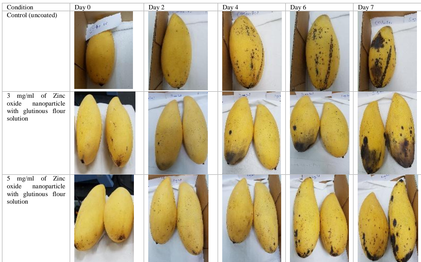
Fig. 1: shows the mango with and without coated with ZnO nanoparticles in several day observation.
