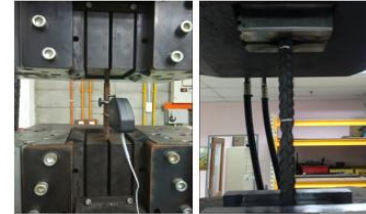
Fig 5(d) Fig 5(e) Steel bar (12mm) coupon before and after failure
