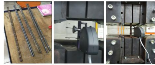
Fig. 5(a) Fig. 5(b) Fig. 5(c) Specimen preparation NiTi bar before and after failure.
