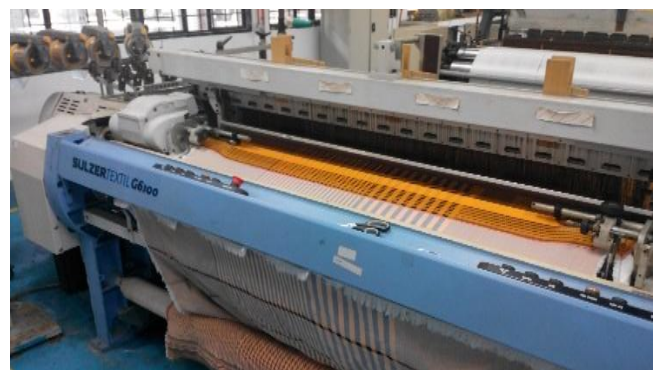
Fig 1: Sulzer Rapier loom located in Textile Weaving Workshop, UiTM Shah Alam.
