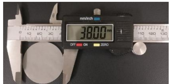
Fig. 2: Geometry and dimensions of the abrasion resistance samples
