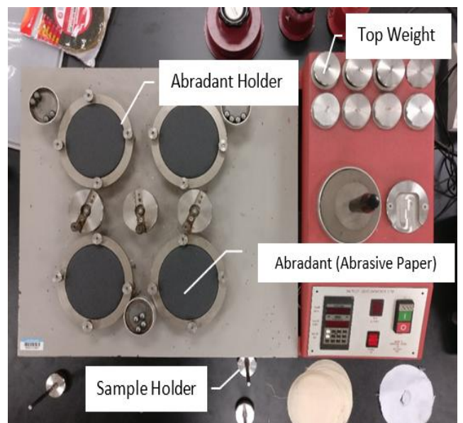
Fig. 8: Abrasion resistance set-up (Without cover)
