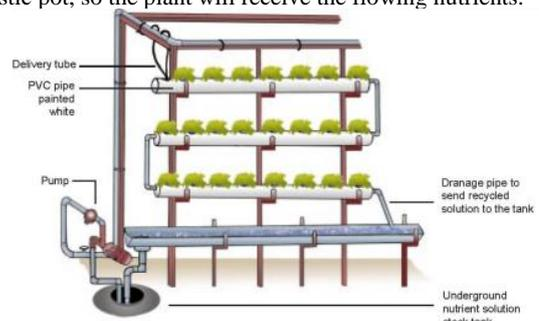
Figure 1. Illustration of Zig Zag DFT System
