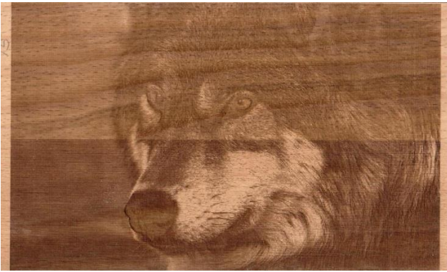
Fig. 1: The engraving obtained on the furniture panel glued from the bars of the wood of one breed; beech; 95x155 mm
