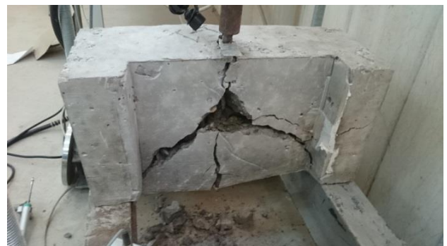
Fig. 15: Side-Face Blowout Mode of Failure in Compression Test.
