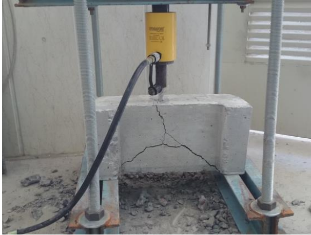
Fig. 16: Shear Related Mode of Failure in Compression Test.
