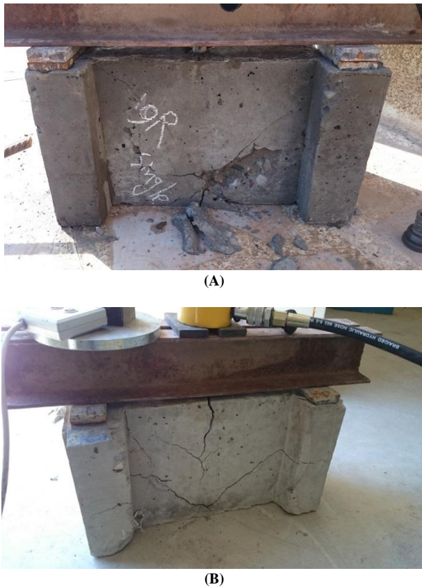
Fig. 9: Failure of Headed Reinforcement in Pullout Tests (A) Single Headed Bar (B) Dual Headed Bar.
