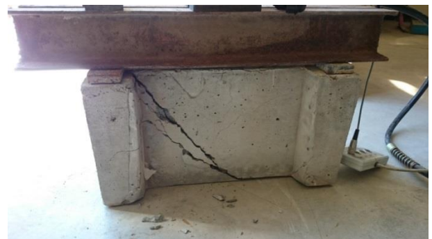
Fig. 11: Sudden Shear Related Mode of Failure.
