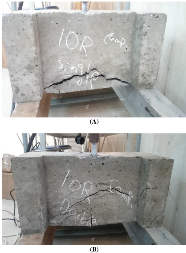
Fig. 12: Failure of Headed Reinforcement in Compression Tests (A) Single Headed Bar (B) Dual Headed Bar.
