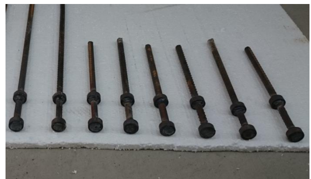
Fig. 2: Dual Headed Bars (A) Circular Heads before Welding (B) Dual Headed Bars after Head Attachments.
