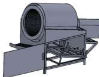
Fig 3: Design Proposal of Frying Machine
