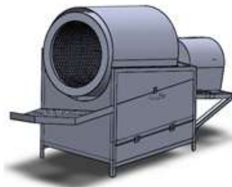
Fig 1: Design Concept of Crackers Frying Machine with Sand Media (Purwitasari, Y. (2015))
