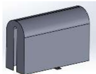
Fig 8: Motor Cover Design Proposal
