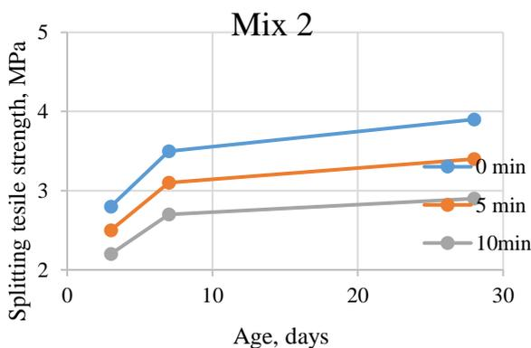
Fig. 6: Splitting tensile strength versus age for various microwaving times
