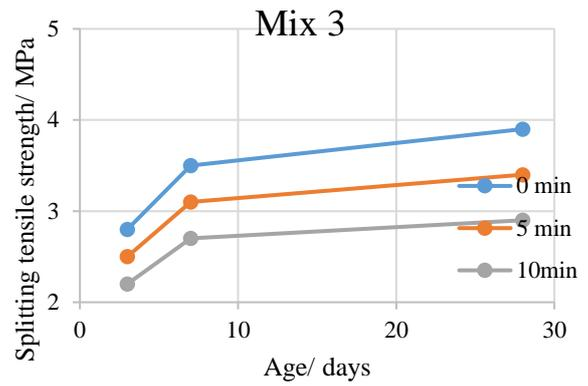
Fig. 7: Splitting tensile strength versus age for various microwaving times
