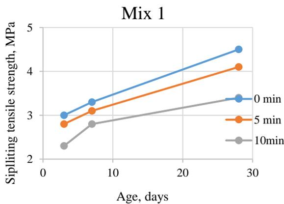
Fig. 5: Splitting tensile strength versus age for various microwaving times
