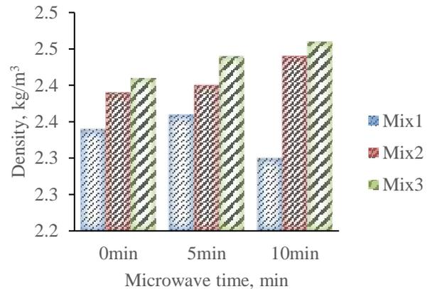
Fig. 7: The density of various SCC mixes
