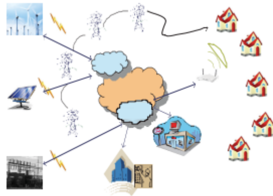
Figure 1: Example of communication architecture in smart grid.
