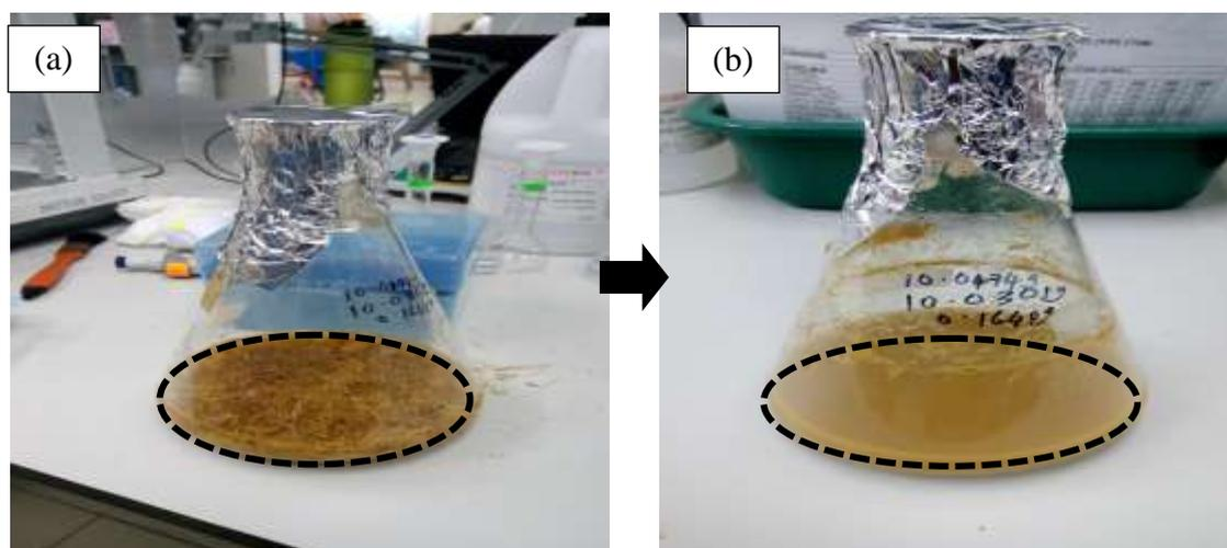
**Fig 6:** (a) shows the sample preparation of the high glucan loading (6%) and (b) the liquefaction obtained after enzymatic hydrolysis process occurred after 72 hours at 30 FPU/g glucan, 45°C and 250 rpm
