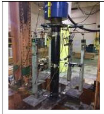
Fig. 3: Test set up of slender circular CFSTC ( $h = 1500$  mm)
