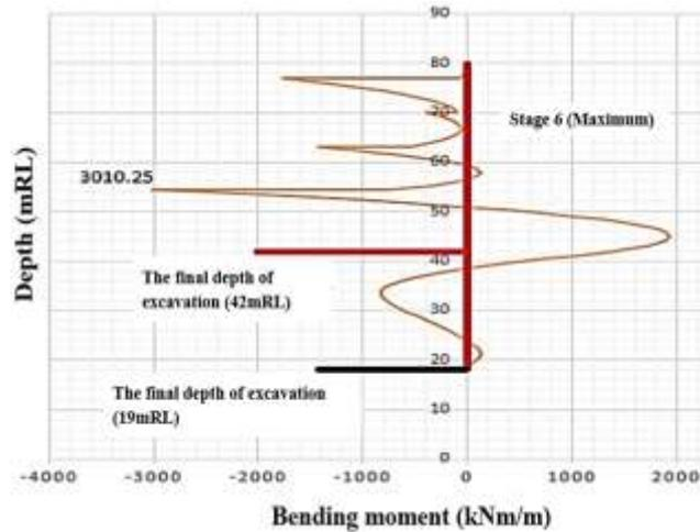
Fig. 6: Bending Moment (Left wall)
