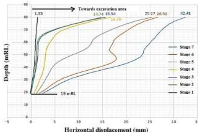
Fig. 5: Horizontal Displacement (Left wall)
