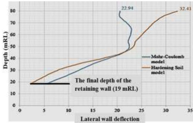
Fig. 3: Effect of soil model (Left wall)
