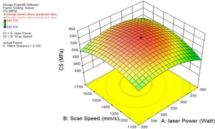
Fig. 10: 3D surface CS vs. laser power and scan speed
