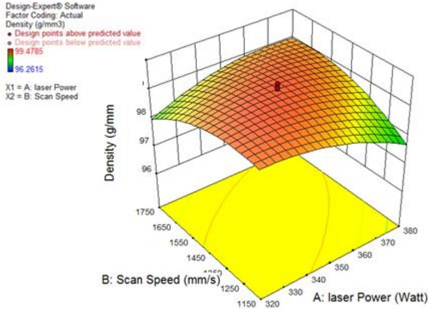
Fig. 7: 3D surface RD vs. laser power and scan speed
