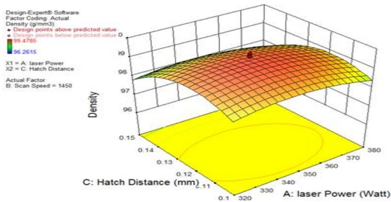
Fig. 8: 3D surface RD vs. laser power and hatch distance
