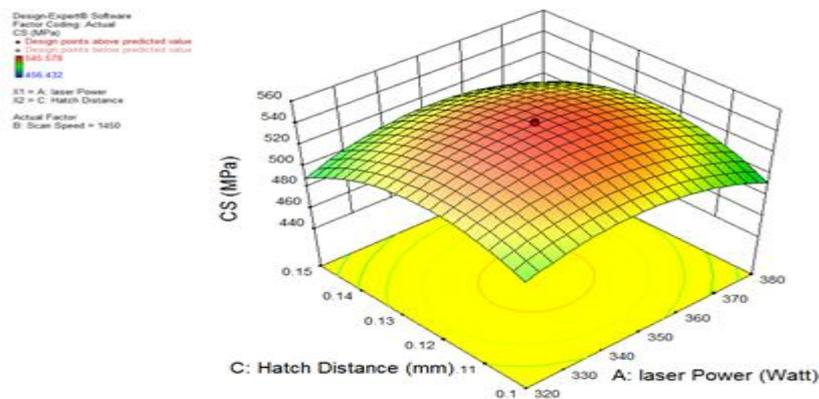
Fig. 11: 3D surface CS vs. laser power and hatch distance
