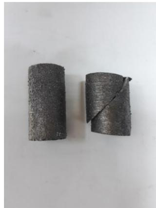
**Fig. 13:** Compression samples before and after testing
