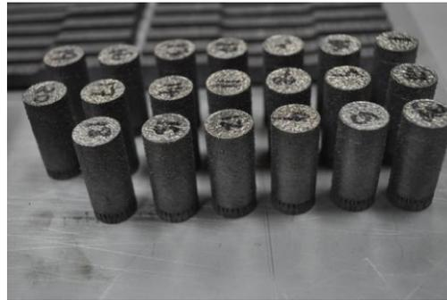
Fig. 2: The compression samples built by the SLM process.
