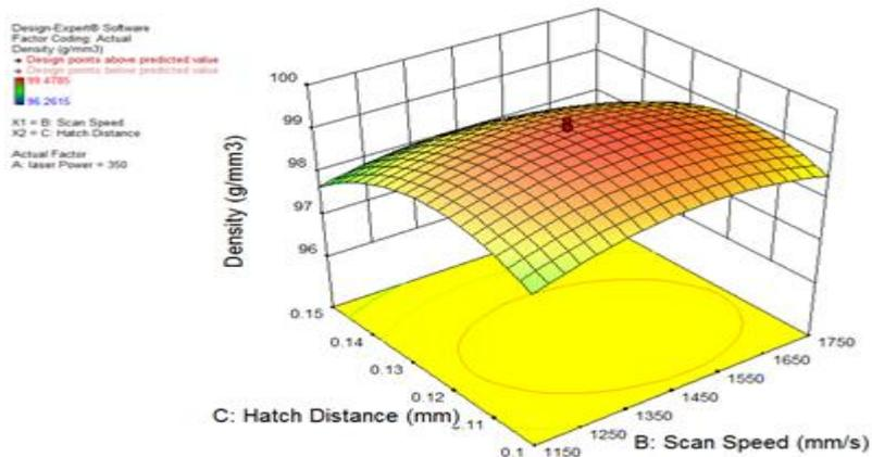
Fig. 9: 3D surface RD vs. scan speed and hatch distance
