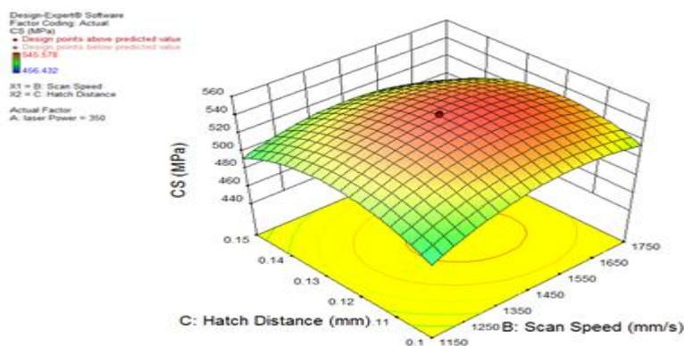
Fig. 12: 3D surface and CS vs. scan speed and hatch distance
