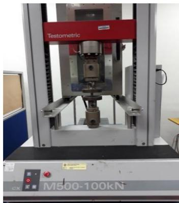
Fig. 1: Testometric M500 compression testing machine
