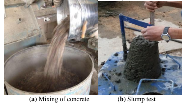
Fig. 2: Photos showing mixing of concrete and the slump test
