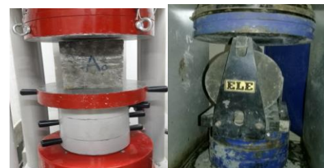
(a) Compression test (b) Splitting tensile test
