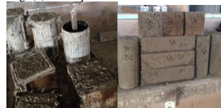
Fig. 3: Photos for specimens during casting and after de-moulding.
