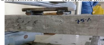
(c) Flexure third point test
