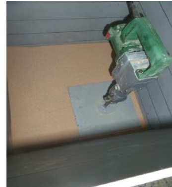
Plate 2: Compacting soil model by modified jackhammer
