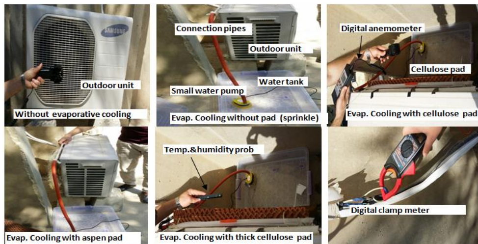
Fig. 1: Illustrates Test Rig, Measurement Apparatuses and Experimental Work.
