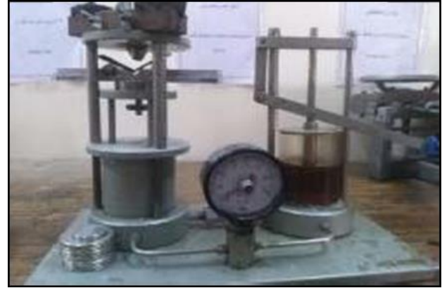
Fig.4 :Flexural test apparatus
