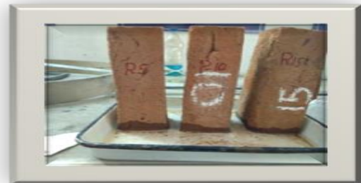
Fig. 3.3: Efflorescence Test on Brick
