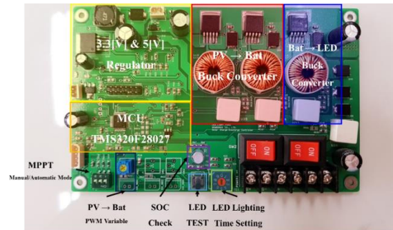
Figure 6: Constant Current Drive System Made using LM2576
