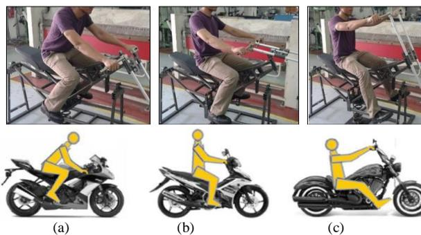
Fig. 2: Common motorcycle riding postures; (a) Forward-lean, (b) Standard upright, and (c) Slightly recline
