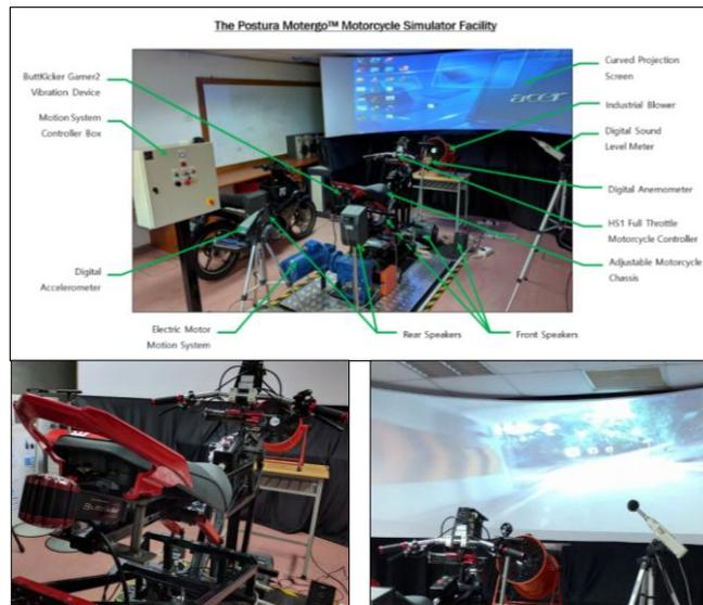
Fig. 1: The Postura Motergo™ motorcycle simulator facility
