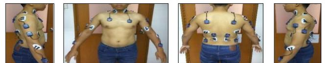
Fig. 3: Electrodes with sEMG transmitters attached at seven bilateral muscle groups
