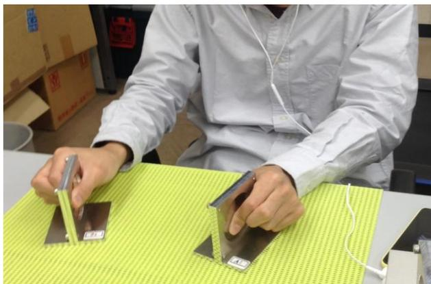
**Fig. 4:** Experimental setup where the test subject is comparing the stimulus between two copper samples with specified thickness.
