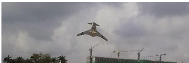
Fig. 3: Extreme pitch up moment during takeoff
