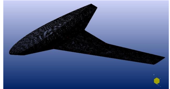
(c) Mesh of the front case
