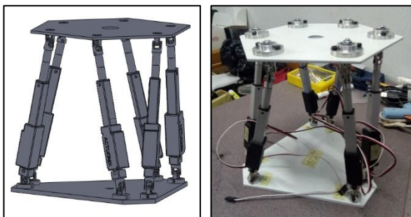
Fig. 26: Illustration of hexapod manipulator design (left) and prototype manipulator (right).
