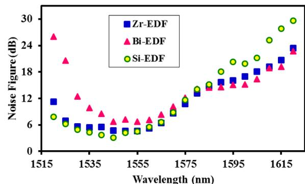
**Fig.4:** Noise figure analysis of -30dBm Zr-EDF, Bi-EDF and Si-EDF
