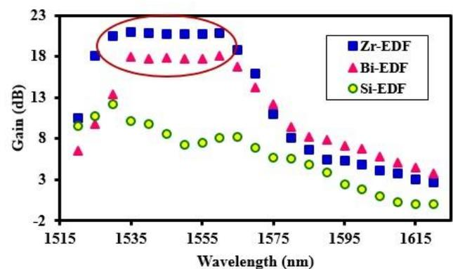
**Fig.3:** Gain analysis of -10dBm Zr-EDF, Bi-EDF and Si-EDF
