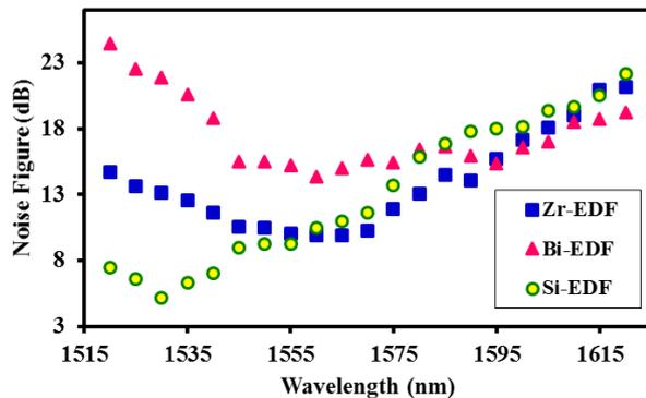
Fig.5: Noise figure analysis of -10dBm Zr-EDF, Bi-EDF and Si-EDF
