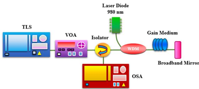
**Fig.1:** Configuration of experimental setup for double-pass optical amplifier by using Zr-EDF and Bi-EDF as gain medium
