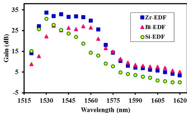
**Fig.2:** Gain analysis of -30 dBm Zr-EDF, Bi-EDF and Si-EDF
