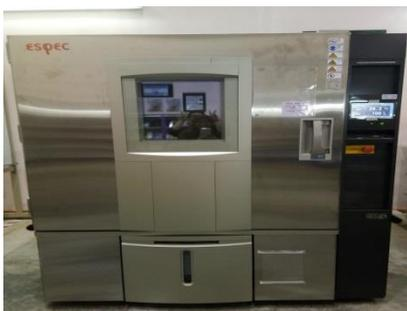
Fig. 5: Temperature (and Humidity) Chamber Platinox J series Equipment
