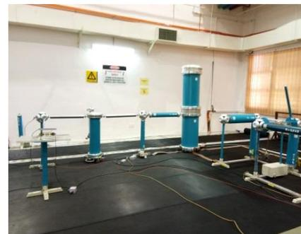
Fig. 3: Setting up for Tan Delta measurement.
