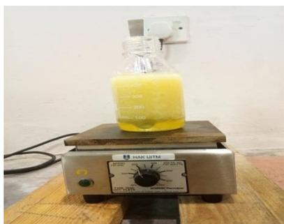
Fig. 6: CPKO had been heated on the hot plate
