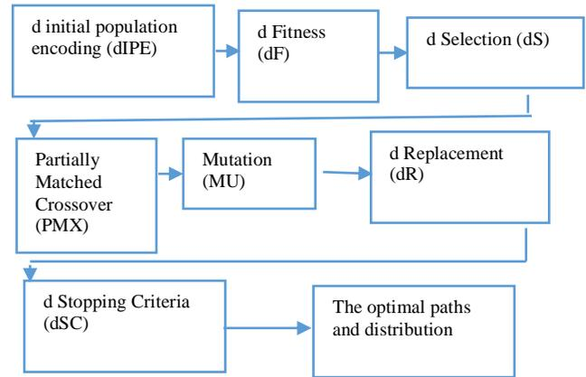
Fig. 2: Major operations of developed genetic algorithm
