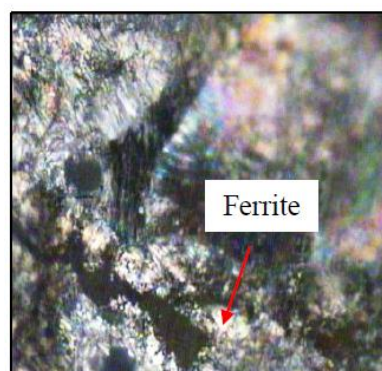
Fig. 3: The microstructure of an as-cast niobium alloyed grey cast iron
