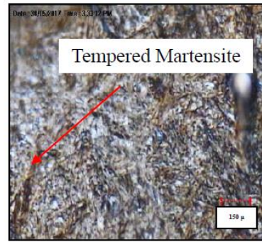
Fig. 6: Structure of tempered martensite
