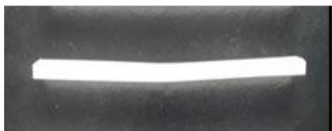
Fig. 7: Flexural testing specimen after 5% max deflection
