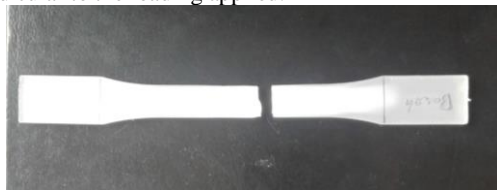
Fig. 3: Tensile test specimen after failure
