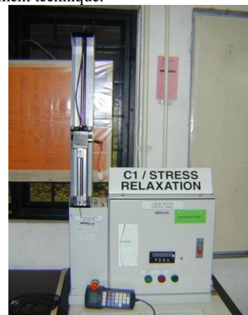
Fig. 1: C1/Stress relaxation machine built in-house
