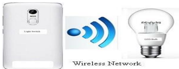
Fig. 1: Set Up Gadget-To-Gadget Connections Through Bluetooth, Z-Wave or Zigbee Can to Switch On/Off A Light Bulb [13].
