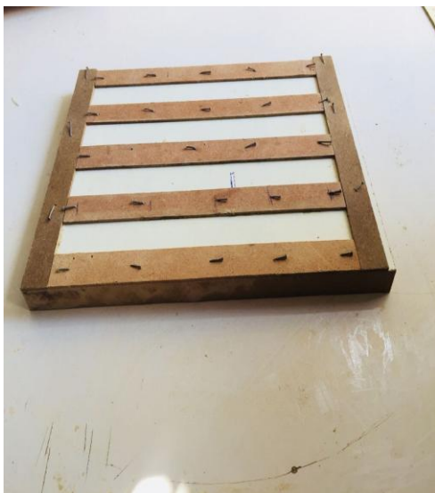
Fig1: Wooden Mould to arrange composite material
