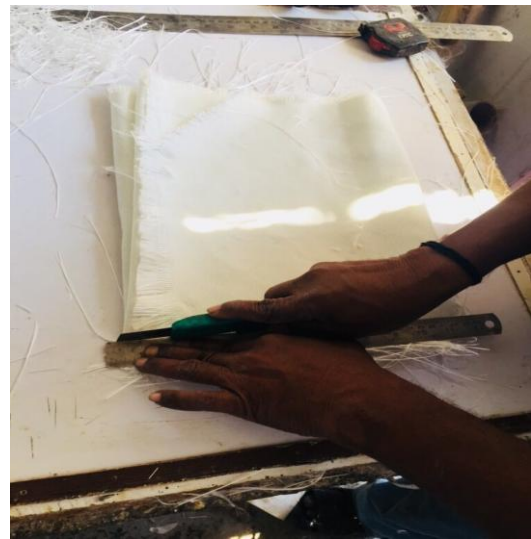
Fig2: Cutting of Glass Fiber
