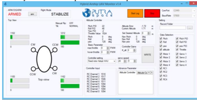
Fig. 18: Hybrid airship UAV monitor software
