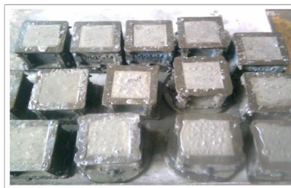
Fig. 5: Casted Cubes of M40 RH Concrete of 10% Replacement.
