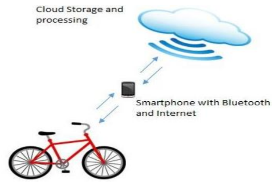
SeB1.0 with: a. In-built accelerometer sensor b. Bluetooth module
