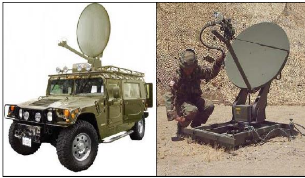
Fig. 11: Satellite DVB-RCS Mobile and Portable Antennas for Military Applications [8].
