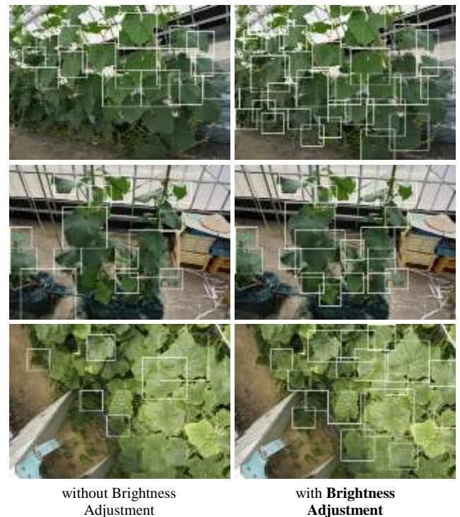
Fig. 6: The improvement of leaf detection in our system with brightness adjustment (right) compared to our previous result without brightness adjustment (left)
