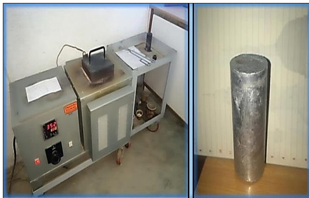
Fig. 1: A) Melting Furnace, B) Ingot of Aluminium Beverage Cans.
