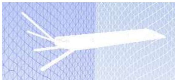
Fig. 8: Computational mesh for flow over a wing with 4 winglets (20°, 10°, 0°, -10°Dihedral)
