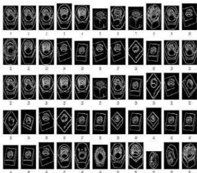
Figure 4.4: Results obtained during edge detection of Hexa and squared nuts
