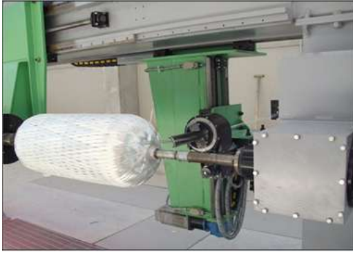
Fig. 2: Filament winding technique
