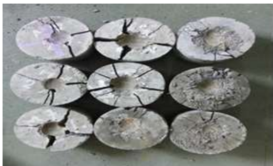
Fig. 11: Impact Strength Test of disc specimen
