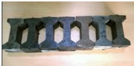
Fig. 2: Dog-Bone shaped specimen
