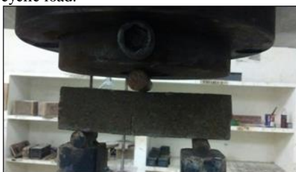
Fig 6: Beams tested for Flexure
