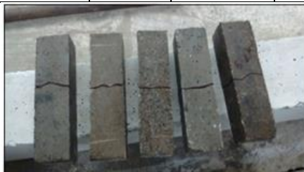
Fig 5: Beams tested for Flexure
