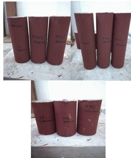
Fig 3: Specimens of Concrete In-filled Mild Steel tube of height 200mm, 300mm and 400mm
