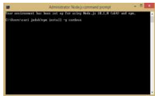
Fig. 4: Cordova installation display
