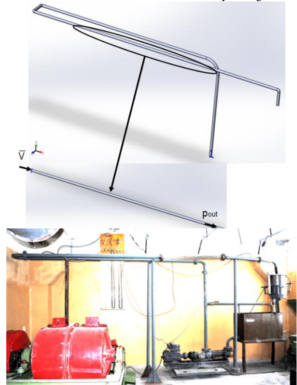
Fig. 1: Three-dimensional model of experimental installation
