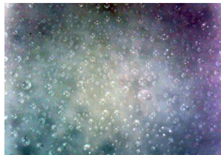
Fig. 5: Picture of fuel drops injected by nozzle T = 300 days after using the fuel supply system clean-in-place technique \Delta_{FL} = 0.998 , \Delta_N = 0.995 (Scale 1:150).
