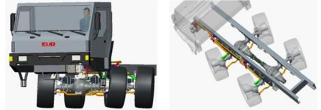
Fig. 4: Three-dimensional model of KrAZ-7634HE with steering linkage.
